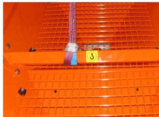
**2.** Type of harness to be made using a cable adequately sized to the weight of the load to be lifted (see Technical Data).
