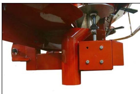
**10.** Position a container with at least 25 liter capacity beneath the deviator tube.**11.** Adjust the hydraulic circuit ball valves as follows (consult the section entitled "Adjustable spreading" on Page 24):
