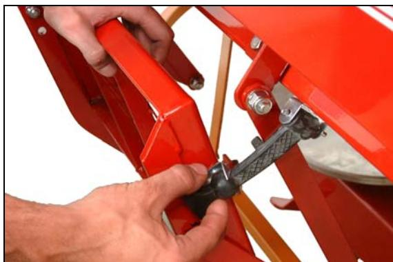
1. Release the fixing rod.
