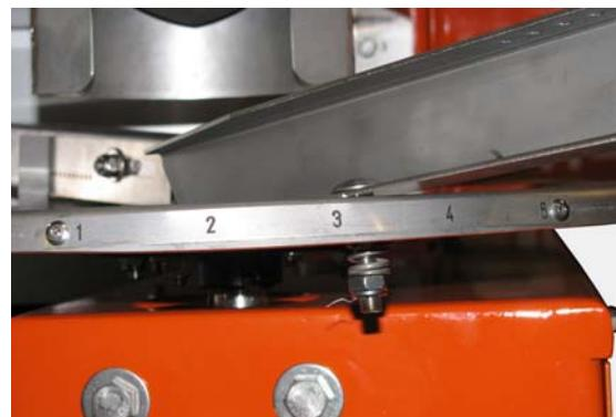
1. Press the disc and pull up the spreading vane.
