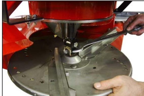
comes completely unscrewed (rotating the shaft clockwise for the left disk and counter-clockwise for the right disk).
