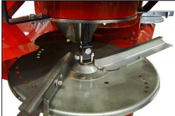
**1.** While keeping the spreading disk held firmly in place, rotate the mixer shaft using an appropriate tool until the disk be-
