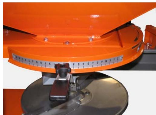
Spreading width adjustment lever.
