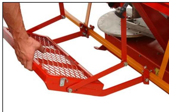
4. After completing loading operations, re-close the loading platform and fasten it in place using the respective fixing rod.
